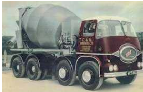
Eight cubic yard High Discharge ERF
